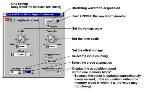
Starting/Stopping waveform acquisition in the digitizer mode and setting the input conditions of the waveform and time scale
